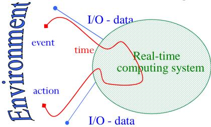
A real-time system is a system that reacts to events in the environment by performing predefined actions within specified time intervals
