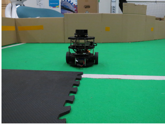
Figure 2: Setup for measuring the noise at different distances in the real world
