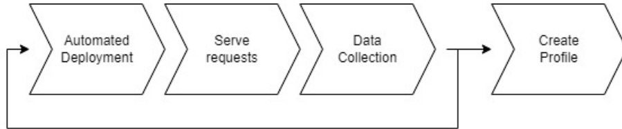
Figure 5.1: High-level workflow of automated profiling framework of an application
